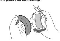
2 Place the new ear pad on the driver unit. Hang the edge of the ear pad on one side of the driver unit's groove edge, then turn the edge of ear pad around the driver unit as illustrated
